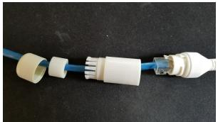
Step 5. Connect everything together and tighten down the compression cup until the barrel gasket is tight around the Cat5 cable.
