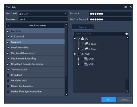
For example, the user "guard" will only have Live View, PTZ Control, Snapshot, Local Recording, Play Local Recordings, Play Remote Recording, Download Remote Recording and Two-way Audio permissions to the two cameras that are selected on the right.
