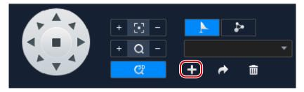
2. On the **Preset** tab, click **Add Preset**. Enter a preset number that is not in use; otherwise, the existing preset will be replaced by the new preset.
