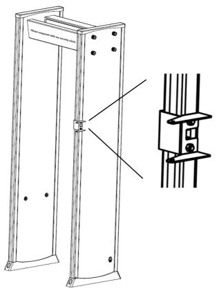
9. Secure the temperature measurement module and the access control terminal to the bracket on the right panel, and then close the junction box.
