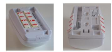
**Step 4:** Clean the mounting surface ideally with rubbing alcohol. Let the surface dry. Press and hold the motion sensor into the corner or wall. Press firmly and hold for at least 10 seconds to ensure a strong connection.
