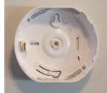
**Step 3**: Place the main sensor onto the base - ensure the three LEDs on the front light up in sequence to confirm the base is properly attached.
