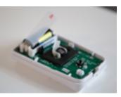
**Step 2:** Pull the battery tab to activate the sensor. For the next 30 seconds the sensor will be in calibration mode and will not detect motion. Place the face plate back onto the sensor.
