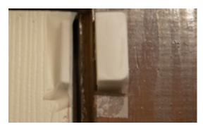
**Step 3**: Once you've selected a good spot - clean the surface area of the door, ideally with rubbing alcohol. Be sure that the surface temperature is above 50 degrees. Dirty or cold surfaces may cause the sensor to fall off, causing a false alarm. After cleaning be sure to let the surface dry before placing sensors.
