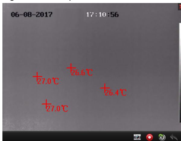
Figure 5-7 Temperature Measurement on Points
